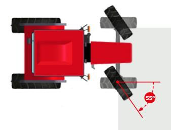
The X6.4 combines wide axle oscillation and high ground clearance with a 55-degree steering angle making for excellent manoeuvrability and driving accuracy in any situation. In addition, the hydrostatic power steering delivers smooth steering control even at low engine rpm. The suspended axle allows a top speed of 50 km/h.
