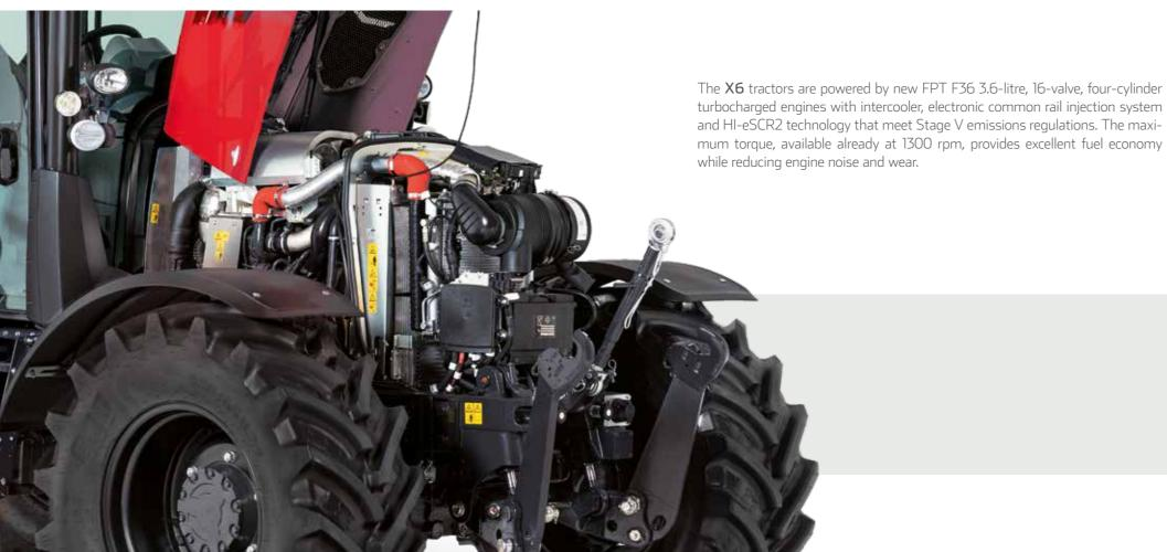
The FPT F36 engine is equipped with an electronic high-pressure common rail injection system that optimises fuel atomisation and combustion, thereby improving engine performance and fuel economy while reducing emissions. Fuel efficiency is further enhanced by the Engine Memo switch, a device that allows the operator to store and
