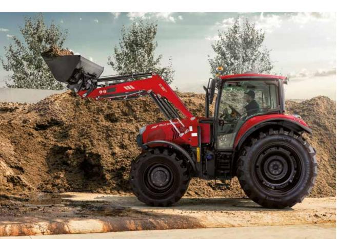
Designed to be integrated into the **X6** tractor, the McCormick M30 front loader is built from HLE (High Limit Elasticity) steel, a material capable of withstanding impressive loads. The M30 front loader is intuitively controlled via the convenient multifunction joystick. The main strong points of the M30 front loader are the following:
