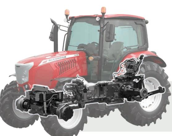
The **X5** features an open-centre hydraulic system with a pump that provides a flow rate of either 62 l/min or 82 l/min to operate the remote valves, the front and rear hitches and the front loader. A second pump with a flow rate of 32 l/min is dedicated to the steering system. This hydraulic capacity allows the operator to:
