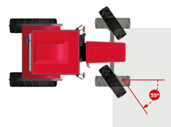
The **X6.4** combines wide axle oscillation and high ground clearance with a 55-degree steering angle making for excellent manoeuvrability and driving accuracy in any situation. In addition, the hydrostatic power steering delivers smooth steering control even at low engine rpm. The suspended axle allows a top speed of 50 km/h.
