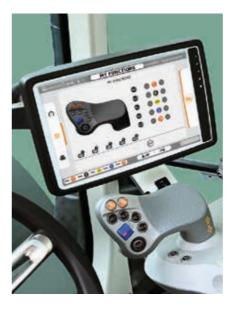
ThenewMvFunctionsmenuprovidesfullvcustomisable control of tractor and implement. allowing the operator to configure and save up to five different functions via the DSM touch screen monitor. All controls have also been ergonomically repositioned on the multifunction armrest to improve comfort and ease of operation.
