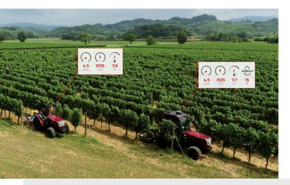
1. Real-time fleet monitoring: The sys- 2. Data analysis: The data coming from by checking parameters like speed, engine take informed decisions. hours and RPMs, fuel and AdBlue levels, average consumptions and work progress.
