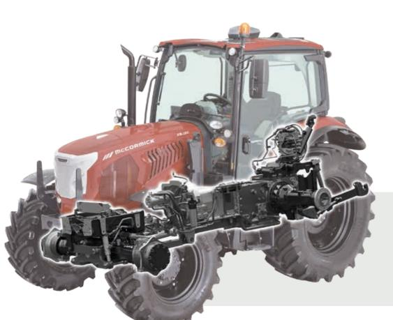
The **X5** features an open-centre hydraulic system with either a dual pump that provides a flow rate of 62 l/min or a triple pump with up to 82 l/min to operate the remote valves, the front and rear hitches and the front loader. A second pump with a flow rate of 32 l/min is dedicated to the steering system. This high hydraulic capacity allows the operator to:
