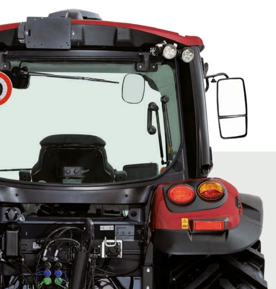
Spacious, quiet, technically innovative and above all comfortable – that's the new Total View Slim cab of the McCormick **X5**. The new cab offers the comfort of two silent-block suspension units at the front and two shock absorbing rubber mounts at the rear for a unique driving experience. This solution cuts down vibrations caused by rough terrain, making for more relaxing and productive work days. Also, a new sound proofing system ensures the cab is completely isolated from exterior noise.
