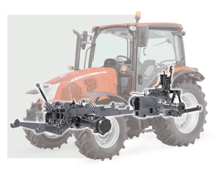
The hydraulic system of the **X4** range features two pumps. One pump provides a flow rate of 30 l/min to the steering system ensuring smooth and precise turning in the field and on the road for enhanced operator comfort and productivity. The other pump supplies 52 l/min to the hitch and remote valves.
