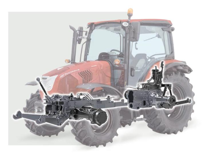
The hydraulic system of the **X4** range features two pumps. One pump provides a flow rate of 30 l/min to the steering system ensuring smooth and precise turning in the field and on the road for enhanced operator comfort and productivity. The other pump supplies 52 l/min to the hitch and remote valves.
