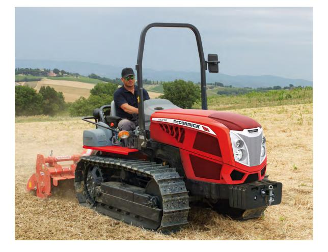
The **TX4** crawler tractor is McCormick's specialist for tough terrains, capable of going where no other tractor can. The **TX4** provides all the traction and grip needed to tackle all types of difficult terrains including steep grades. The **TX4** comes in two versions: **TX4 F** for vineyard and orchard work and **TX4 M** for hillside operation.
