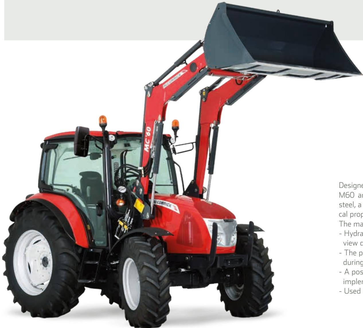
Designed to be integrated into the X4 Series tractor range, the McCormick M60 and M80 front loaders are built from HLE (High Limit Elasticity) steel, a material capable of withstanding high loads thanks to its mechanical properties.
