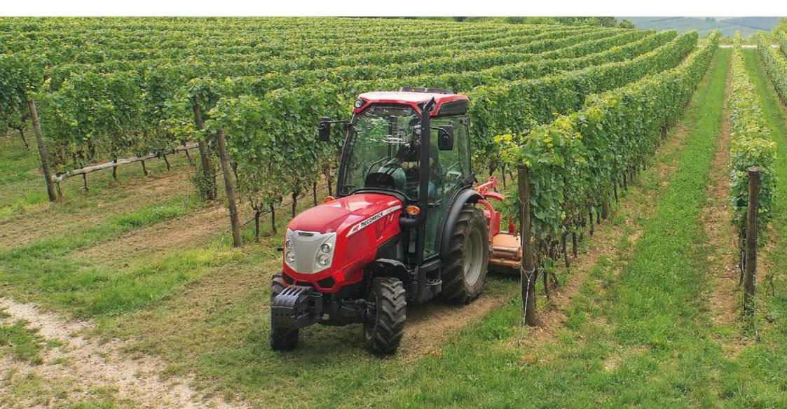
The X4V is McCormick's new specialty vineyard tractor. All five models in the range are powered by the new Deutz TCD L4 2.9L, 4-cylinder engines that cover maximum power outputs from 70 to 102 hp at 2200 rpm. All engines meet Stage IIIB / Tier 4 Interim emissions standards and are equipped with exhaust gas recirculation system (EGR), diesel oxidation catalyst (DOC) and Engine Memo Switch to store engine rpm. These tractors feature a 80L fuel tank for extended run-times without refuelling.
