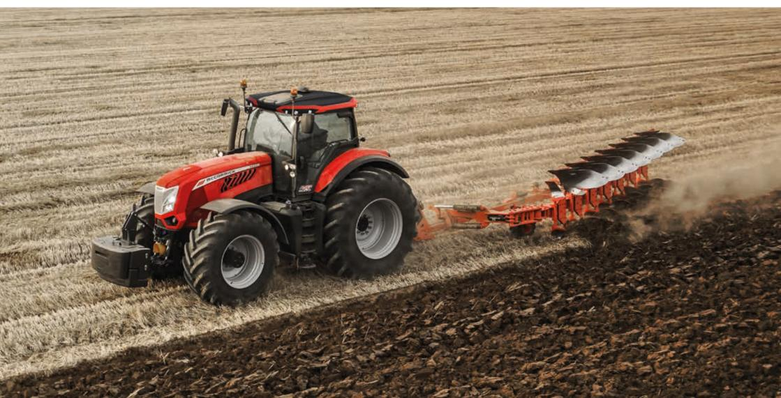
The new X8 VT-Drive series is the top of the range in McCormick tractor line-up. Boasting over 300 hp, the new X8 VT-Drive meets Stage V emissions regulations. The new tractor sports a refreshed look that includes a new cab roof with up to 12 work lights to improve night-time visibility.
