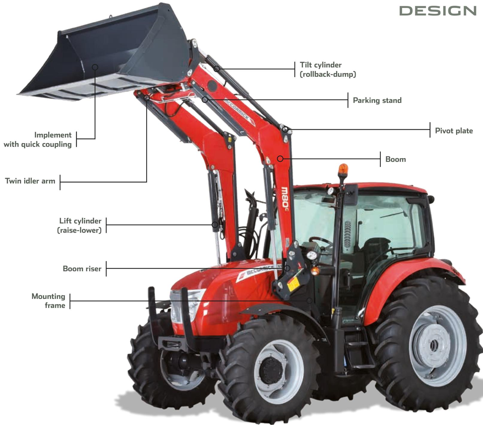
McCormick front loaders are equipped with Euro implement holder enabling the use of a wide range of implements (fig. A).
