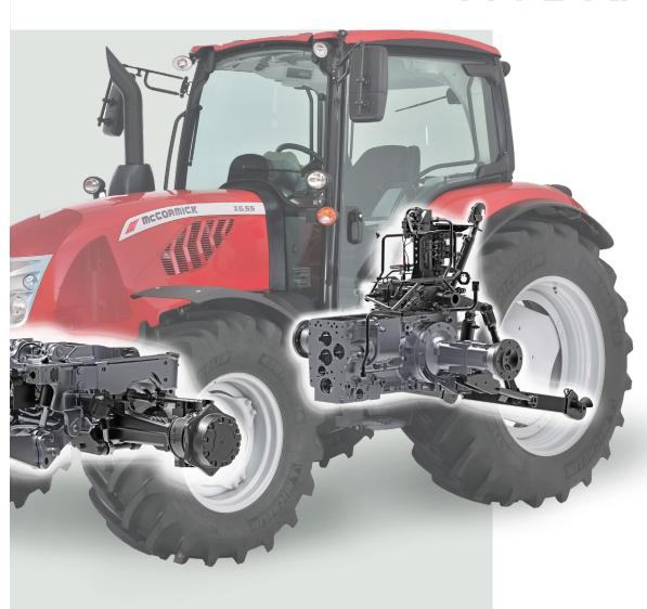
The **X6** standard series features an open-center hydraulic system with a total flow of 24.3gpm (92 lpm) allowing efficient operation of all hydraulic functions. A dedicated pump supplies 16.4 gpm (62lpm) to the rear remote valves and 3 point hitch, while a separate gear pump supplies 7.9gpm (30lpm) to the steering system ensuring smooth and precise turning in any conditions for enhanced operator comfort and productivity.
