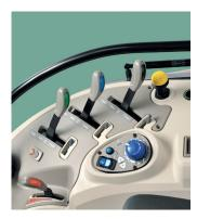
The **X6 standard** comes equipped with three remote valves mechanically operated by levers on the right-hand console. High-quality quick-release couplings allow quick and easy connection/disconnection of hydraulic lines for fast operation.
