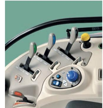
The **X6 standard** comes equipped with three remote valves mechanically operated by levers on the right-hand console. High-quality quick-release couplings allow quick and easy connection/disconnection of hydraulic lines for fast operation.
