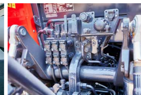
CLOSED CENTRE HYDRAULIC SYSTEM
