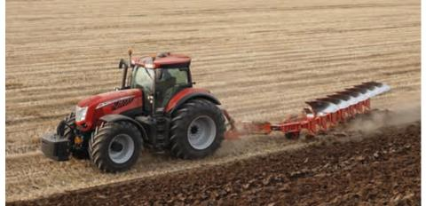
cated menu included in the 12-inch DSM touch screen monitor. Standard equipment also includes a front hitch with a lift capacity of 5000 kg, while a front 1000rpm-PTO is supplied as an option. The front axle is equipped standard with an electronically-controlled centre-pivot suspension system and wet multi-disc brakes to ensure safe positive stopping and driving comfort.
