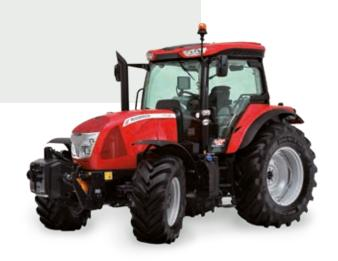
McCormick X6.4 is available in 3 models featuring 121 HP, 133 HP and 140 HP power ratings, 4-cylinder 4500 cc Betapower Fuel Efficiency emissionized STAGE 4 / TIER 4 FINAL engines with SCR + DOC exhaust gas aftertreatment system and with a VT-Drive 3-stage continuously variable transmission manufactured by Agro Tractors.
