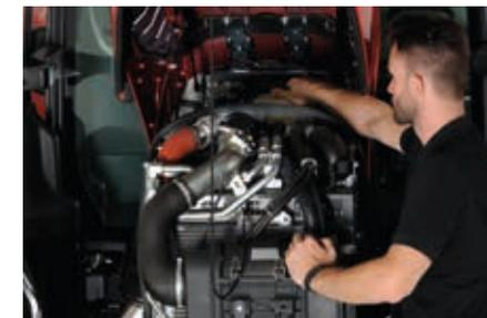
Designed to deliver maximum efficiency and reliability, the **X6.4** range offers a variety of solutions to simplify and expedite maintenance. For example, the tilt-up hood is designed to open wide to provide easy access to the engine compartment for service and maintenance.
