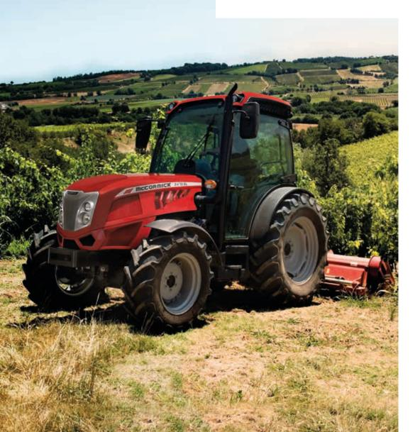
The **X4F** tractors feature as standard a Speed Four modular transmission with four synchronized gears and three ranges that provide 12 forward and12 reverse speeds. Transmission options include a Power Four module (Hi-Lo splitter) providing 32 forward and 32 reverse speeds, an Xtrashift three-stage powershift (high-medium-low) giving a total of 48 forward and 16 reverse speeds, and a creeper that provides speeds as low as 300 m/h at maximum engine rpm.
