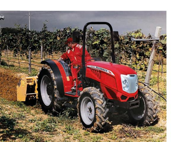
The ROPS version of the X4F features as standard a Speed Four transmission with four gears and three ranges providing 12 forward and 12 reverse speeds with synchro shuttle. A 15+15 Speed Five transmission with five gears and three ranges with either synchro or power shuttle is available as an option.
