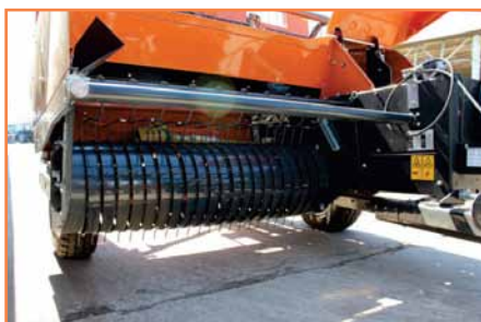
SPRING LOADED PICK-UP WITH FLARED INTAKE
