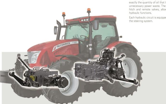
The X7 series tractors feature a closed-centre hydraulic system with variable-displacement pump. This means that the pump always delivers exactly the quantity of oil that the system requires, thereby eliminating unnecessary power waste. The system supplies up to 160 l/min to the hitch and remote valves, allowing for simultaneous operation of all hydraulic functions.
