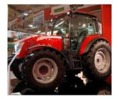
**McCormick X4.50 01a.jpg** A new 'baby' McCormick for livestock farms will span 61hp to 101hp and offer a choice of specification levels to suit different users.
