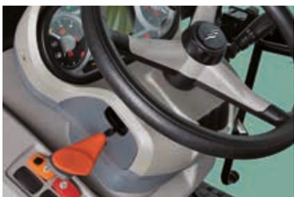
**INVERSOR MECÁNICO O ELECTROHIDRÁULICO**
