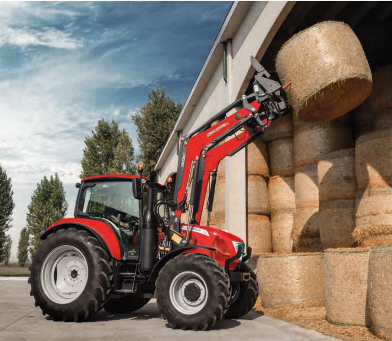
Designed to be integrated into the **X6** Series tractor range, the McCormick M80 and M100 front loaders are built from HLE (High Limit Elasticity) steel, a material capable of withstanding high loads thanks to its mechanical properties.
