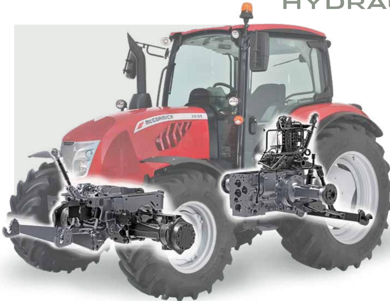
The **X6** Series features an open-centre hydraulic system with a total flow of 66 l/min allowing efficient operation of all hydraulic functions. An 11-litre auxiliary oil tank is optionally available for implements requiring a large quantity of oil. A dedicated pump supplies 30 l/min to the steering system ensuring smooth and precise turning in any conditions for enhanced operator comfort and productivity.
