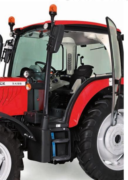
A spacious environment, a flat-deck platform, an efficient sound insulation, an automotive-grade fit and finish, a steering wheel that tilts with the instrument panel, ergonomically-arranged controls: the Deluxe Slim cab is designed to offer the operator maximum comfort and ease of use, making long working days in the field less tiring and stressful. The climate control system, conveniently built into the low-profile cab roof, maintains a comfortable working environment whatever the outdoor
