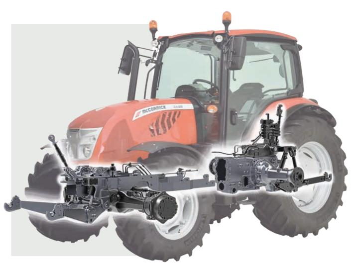
The hydraulic system of the **X4** range features two pumps that provide a standard flow rate of 32 + 44 l/min. One pump supplies oil to the steering system ensuring smooth and precise turning in any conditions for enhanced operator comfort and productivity. The other pump operates all hydraulic functions. A high-flow hydraulic system with dual pump providing a flow rate of 32 + 57 l/m is available as an option. The 2.9L models feature a dual pump with 28 + 49 l/min that covers most
