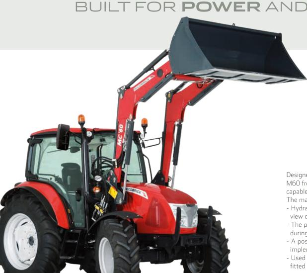
Designed to be integrated into the **X4** Series tractor range, the McCormick M60 front loaders is built from HLE (High Limit Elasticity) steel, a material capable of withstanding high loads thanks to its mechanical properties. The main strong points of the M front loaders are:
