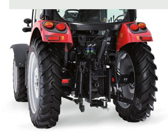
The **X4** tractor range is completely customizable to suit each farmer's specific needs. Thanks to its versatility, it can be simultaneously fitted with either a mechanically- or electronically-operated rear hitch as well as with a front hitch and PTO or a front loader for enhanced productivity.
