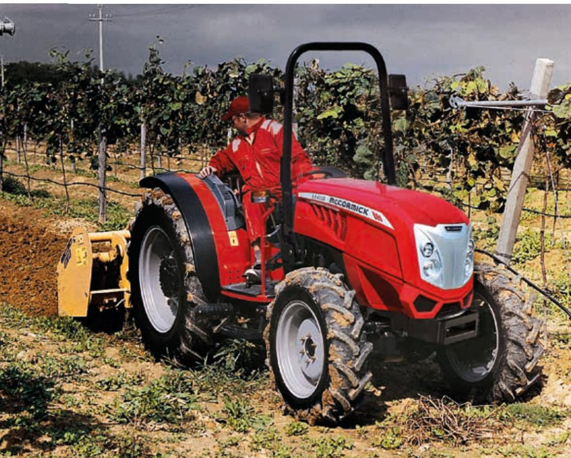
The ROPS version of the **X4F** features as standard a Speed Four transmission with four gears and three ranges providing 12 forward and 12 reverse speeds with synchro shuttle. A 15+15 Speed Five transmission with five gears and three ranges with either synchro or power shuttle is available as an option. The Speed Five transmission can be combined with a Power Five module to obtain up to 30 forward and 30 reverse speeds. A creep speed option is available for all versions.
