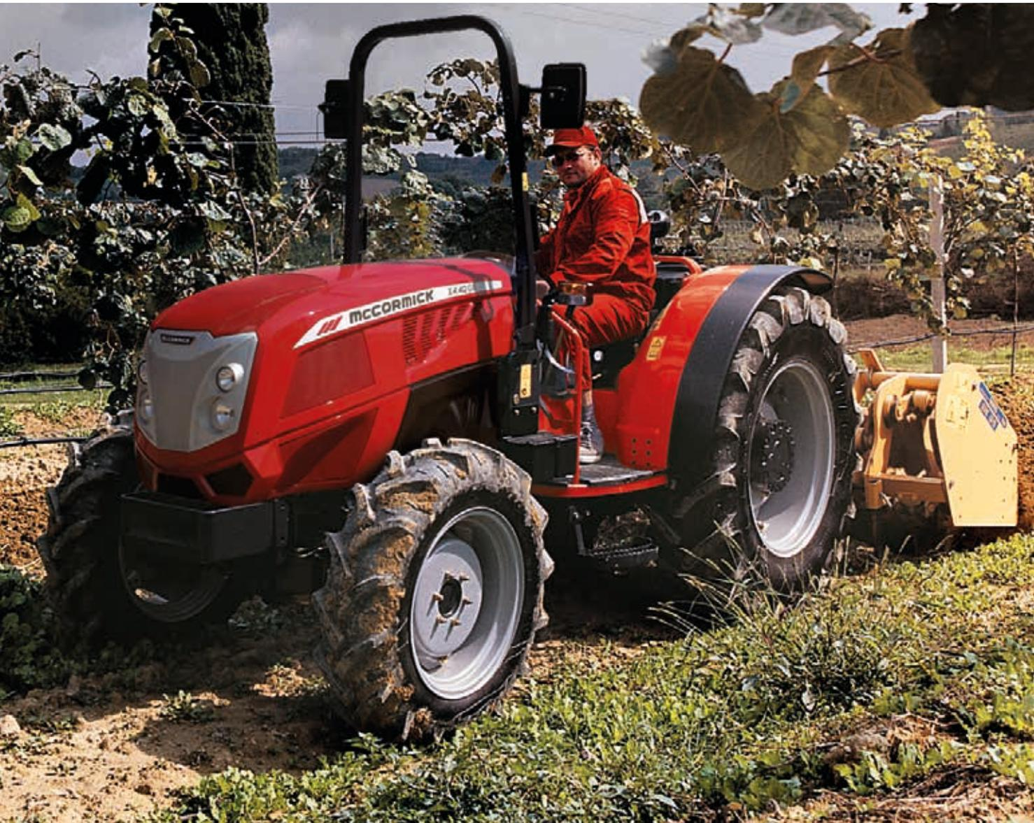
The ROPS models feature as standard a hydraulic system with a double pump that supplies 50 l/min to the rear hitch and remotes and 28 l/min to the steering system. Available as an option is a triple pump that provides a flow rate of 44+41+28 l/m to operate, respectively, the rear hitch and remotes, the front remotes and the steering system. Three mid-mounted front remotes are available on request with the triple pump in combination with a joystick for the control of front-mounted implements.
