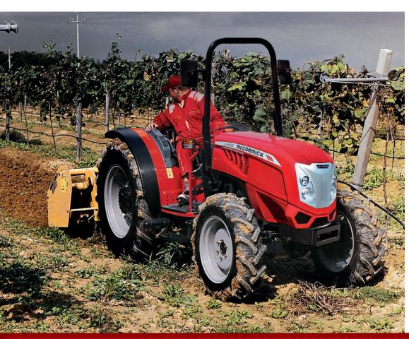
The ROPS version of the X4F and GE features as standard a 16x16 speed transmission with creeper gear and synchronized mechanical shuttle capable of 25mph (40kph). A 15x15 speed transmission with five gears and three ranges is available with reverse power shuttle. This five gear transmission can be optionally combined with 2-speed power shift and creeper reduction gears to obtain 40 forward and 40 reverse speeds.
