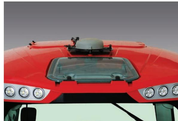
The automatic climate controls are conveniently built into a stylish roof console. An opening transparent roof hatch provides extra visibility for loader operations.
