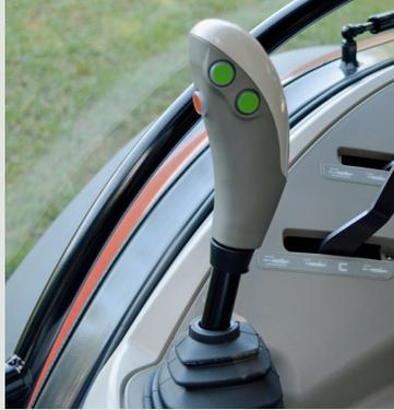
X5.40 and X5.50 models are available with 3-speed powershift option that gives operators the ability to quickly upshift and downshift through 3 power shift gears using 2 buttons integrated into the main transmission lever.
