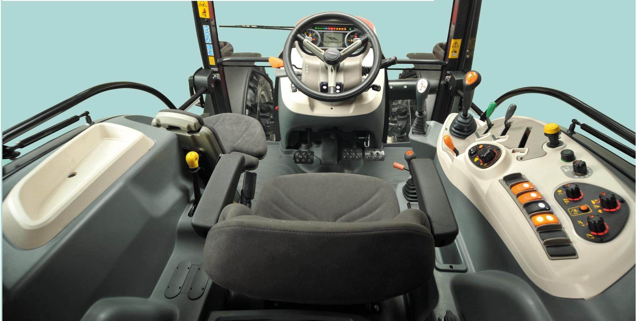
The McCormick X5 sports a large 4-post cab with completely flat foot deck and twin opening doors for easy entry and exit. The deluxe air-suspended seat is fully adjustable for complete operator comfort. The large glass windows and doors provide 360 degrees of visibility and the roof window allows maximum visibility of raised loader buckets. The HVAC system boasts twin blowers to keep the sealed environment of the cab comfortable in all climates.
