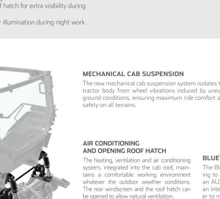
The new mechanical cab suspension system isolates the tractor body from wheel vibrations induced by uneven ground conditions, ensuring maximum ride comfort and
