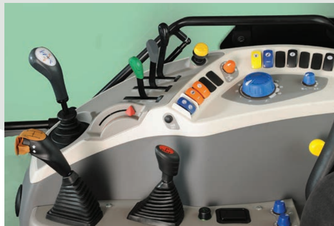
Most major tractor controls are integrated into the right hand console within easy reach of the operator. Positioned for quick identification and simple operation, the intuitive layout ensures maximum productivity.
