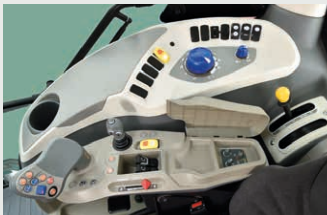
Cab interior on version with VT-Drive transmission: tractor controls are placed on the right armrest of the driver's seat.
