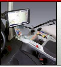
DATA SCREEN MANAGER (DSM) AND MULTI-FUNCTION ARMREST The modern 12-inch DSM touchscreen monitor is bright and provides easy and intuitive control of tractor functions. The multi-function armrest integrated into the seat frame accommodates the main tractor controls.
