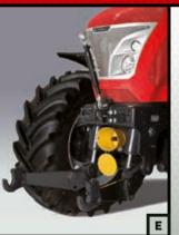
**FRONT HITCH AND PTO** A front hitch and PTO are available as an option to add greater versatility to the tractor for applications using front-mounted implements and rear and front implement combinations (fig. E). When not in use it can be folded to reduce overall length. Control switches at the front allow the operator to raise and lower the hitch for easier implement hook up.
