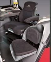
**DRIVER SEAT AND HIDE-AWAY BUDDY SEAT** The driving position features a large and stylish air-suspended driver seat that can be optionally equipped with heating and ventilation system. Passengers can also travel in comfort thanks to an innovative, upholstered buddy seat, which neatly folds away to allow easier and safer access to the cab. The in-cab storage compartment to the left of the operator is air-conditioned..
