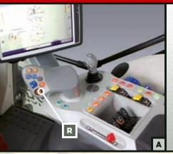
**VT EASY PILOT MULTI-FUNCTION CONTROLLER** An ergonomically-designed controller named VT Easy Pilot (fig.A) integrated into the right-hand armrest provides easy and intuitive control of the VT-Drive transmission allowing the operator to shift through the four speed ranges by simply using his thumb and forefinger without depressing the clutch and the accelerator pedal. The VT Easy Pilot controller features two orange buttons with the
