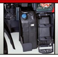
ADBLUE® TANK The Adblue® tank holds 38-litres of fluid for the SCR system which represents the best solution to meet the Tier 4 Interim emission standards.
