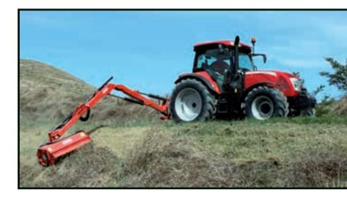
The main technical features of the X6 range include a new 36+12 Xtrashift transmission with a three-step powershift, an electronically-controlled rear hitch with up to 5400 kg lift capacity, an optional 4-speed PTO and an upgraded hydraulic system, which is offered either in standard configuration with a flow rate of 66 l/min or in closed-centre version (LS) with 110 l/ min flow rate.
