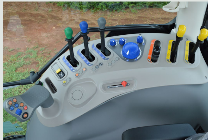
X7 Pro Drive models available in standard configuration feature our efficient cab with multi-function controls integrated into the right-hand console featuring mechanical valve controls.
