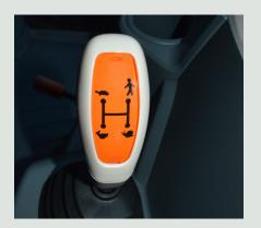
**X5.40** and **X5.50** models available with factory creeper gear set. Located as a 4th position on the range lever, the creeper is ideal for special applications that require the tractor to operate at high RPM's with very low ground speed (0.24 mph / 0.39 kph)
